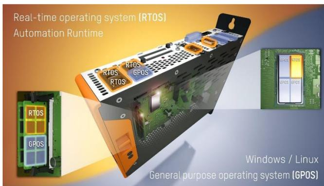
The RTS hypervisor allows all of the hardware resources of an industrial PC to be allocated unambiguously.
